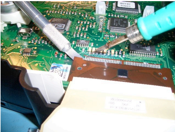
Figure 8: Working with the unsoldering device
