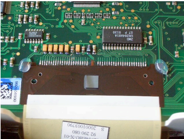
Figure 14: Flat cable soldered on
